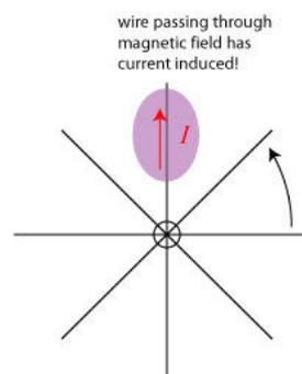
Each wire is passing through a changing magnetic field when it passes the poles of the magnet, and an electric field is therefore induced in the wire! A quantitative assessment of such problems are now regularly assigned in undergraduate electromagnetism courses.
