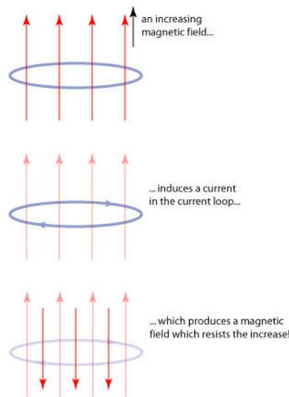
Faraday's law is the basis for one of the fundamental electrical components, the [inductor](#), which in its simplest form is a helical coil of wire. When the amount of current running through the wire is changed, this changes the magnetic field running through the center of the helix. In turn, a counter-current is produced by Faraday's law which resists the original change:
