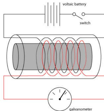
By sending a current through one helix (the black one), Faraday hoped to induce a detectable current through the other (the red one), which he could detect via the galvanometer. His results were not exactly what he expected, however:
