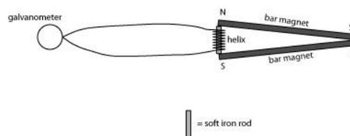
When the bar magnets are touched to the iron rod, it is magnetized! This magnetization of the iron is an increase in magnetic flux, which results in a current appearing in the helix which partially counteracts this magnetization. When the bar magnets are removed, the magnetization was removed, and a current appears in the helix which partially counteracts this demagnetization.
